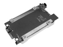
Step 5 Mount the board to the bottom cover.
